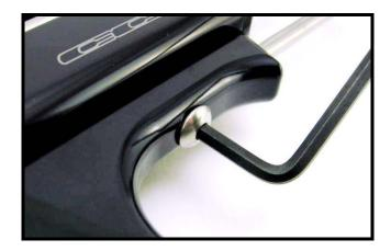
4. Remove the Auto Trigger Arm and Cam from the .45 frame. Sometimes you can simply rotate the AT arm to remove it - if it feels stuck you will most likely have to back out the undertravel screw (see below).
