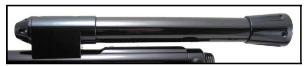
If you are lucky enough to have a Stock Class Feed Assembly, congrats because they are rare. The whole assembly only has three screws and two threaded parts. All three screws ar 5/64<sup>th</sup>.
