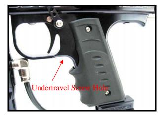
Pump the marker until you hear the sear 'click'. Holding the pump in this position adjust the undertravel screw until it touches the trigger.
