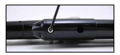
2. Remove both of the hidden screws that attach the feed to the body of the SS 25.
