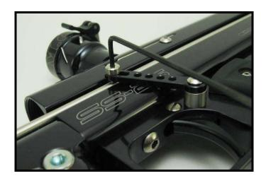
2. Remove the grip panels screws (4 - 5/64<sup>th</sup>) and the grip panels.
