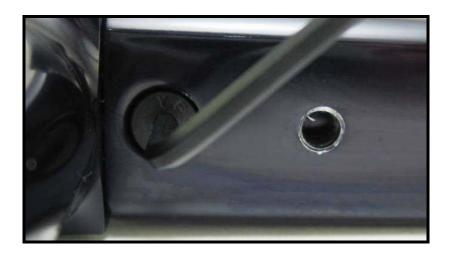
5. Slide the front block out of the marker use great care. There are two orings on the shaft of the front block that can be damaged by the two screw holes they must pass by. When you get the front block out – the valve pin and spring will come out the front.
