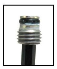
10. Insert the wooden dowel into the rear of the marker and slowly push the valve out of the front of the marker. Again, this valve body has two o-rings on it that can be damaged. Go slow and be careful.
