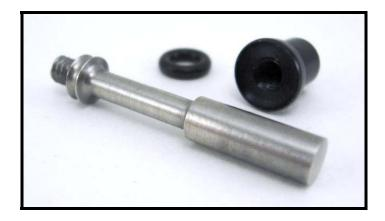
The valve seal is a modular unit that can be taken apart and only the o-ring needs to be replaced. The Valve Pin and Valve Base (Top Hat) are held together with Blue Loc-tite and heat may assist in disassembly. Use Blue Loc-tite upon reassembly.
